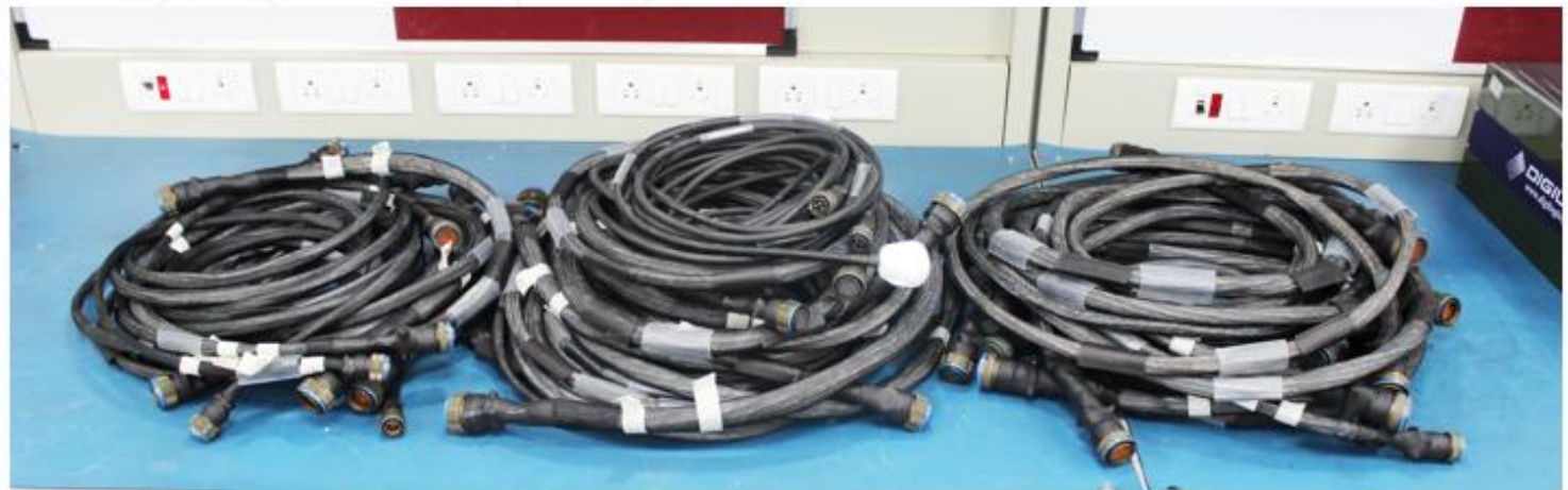
Fabrication of Cable Harness
